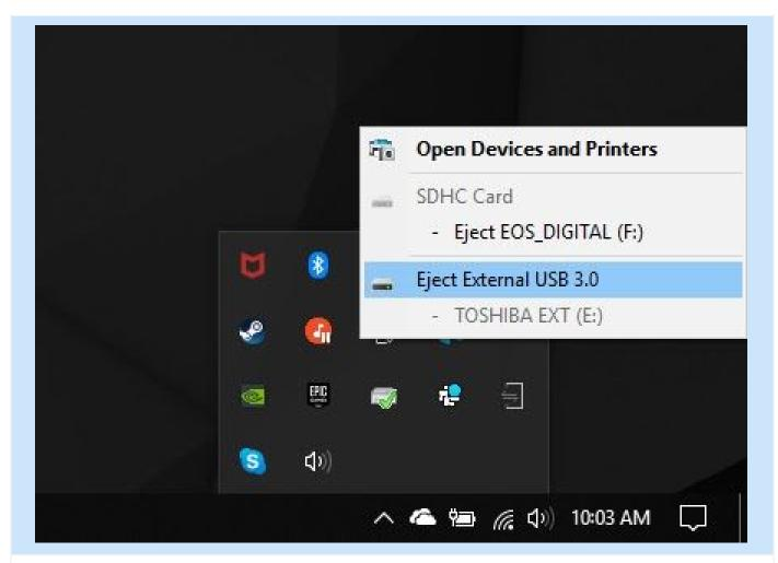
Disconnect the USB drive when done. You can right-click on the drive's icon in Explorer and select "Eject." After doing this, physically remove the external drive by pulling on it gently.
