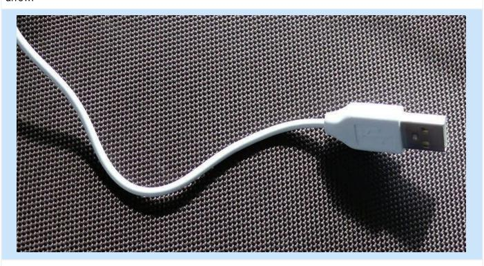
Plug the USB cord into your USB port. The connector should fit easily and snugly into the port; it will only fit in one (01) direction, so flip the connector around if the fit seems wrong.
