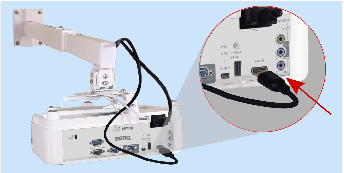
Step 02: Insert HDMI pin in to the Project HDMI Port
