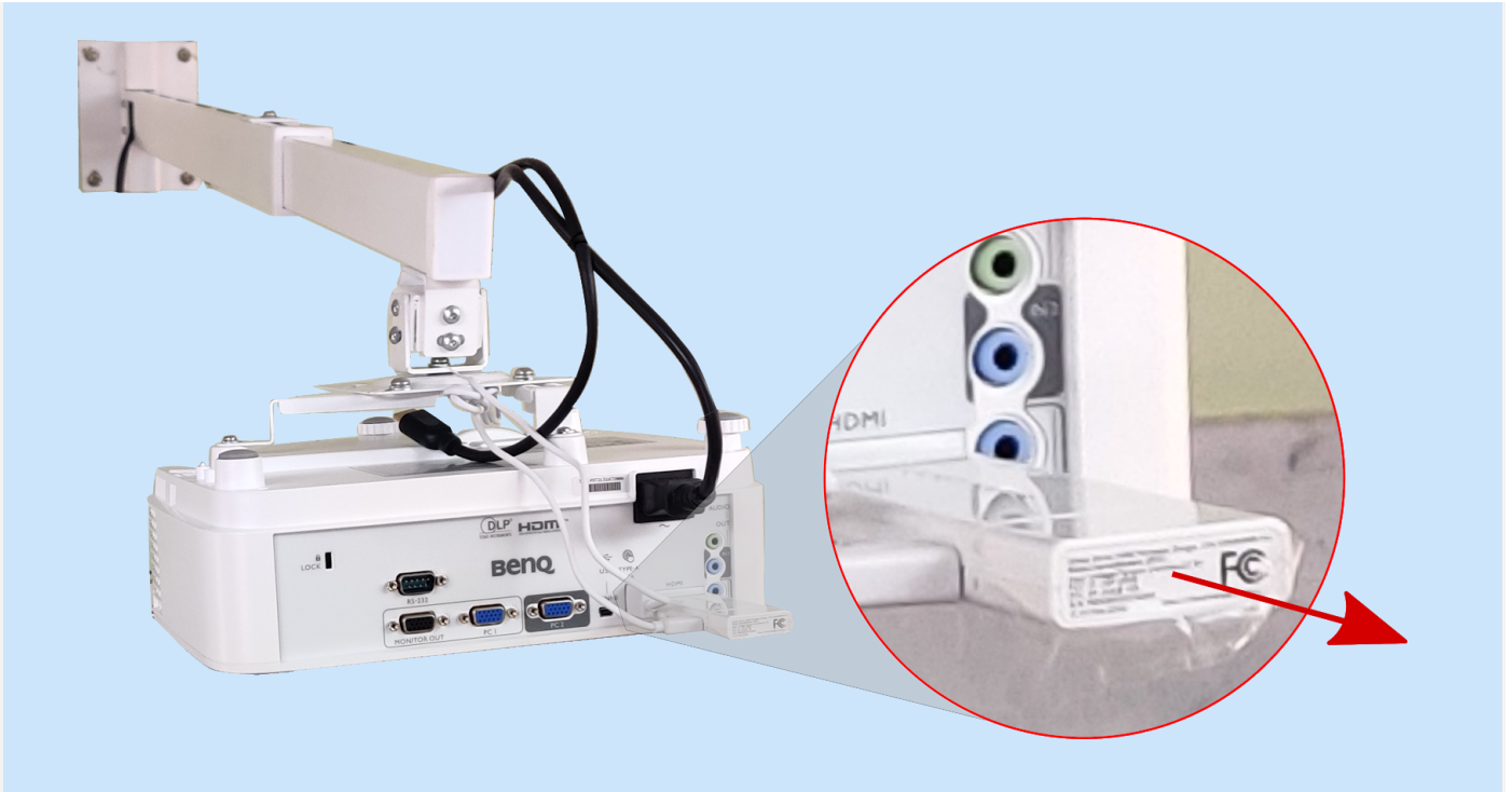
Step 01: Remove Wireless Dongle from the Projector
