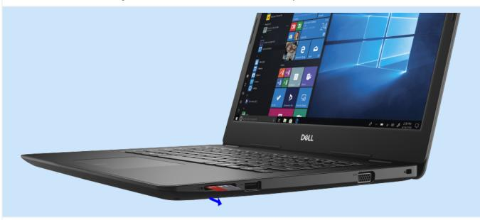
Push the micro secure digital card to release it from the Laptop and slide the micro secure digital card out of the Laptop
