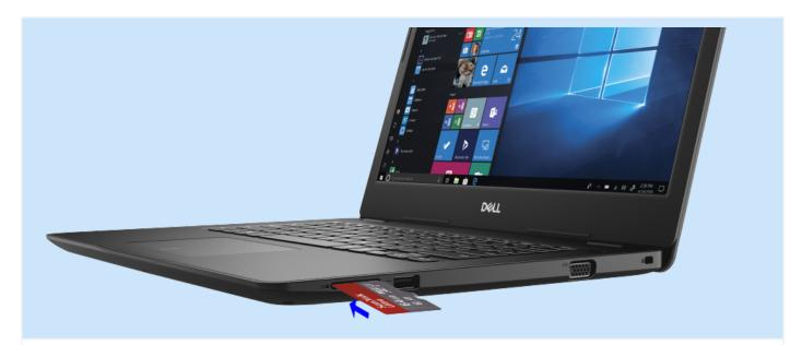
Slide the micro secure digital card into the slot until it locks in place
